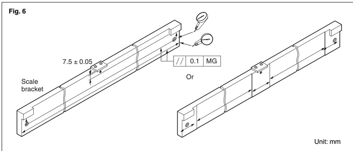
2. Check and adjust the height and parallelism of the slider bracket, and then secure in place.
