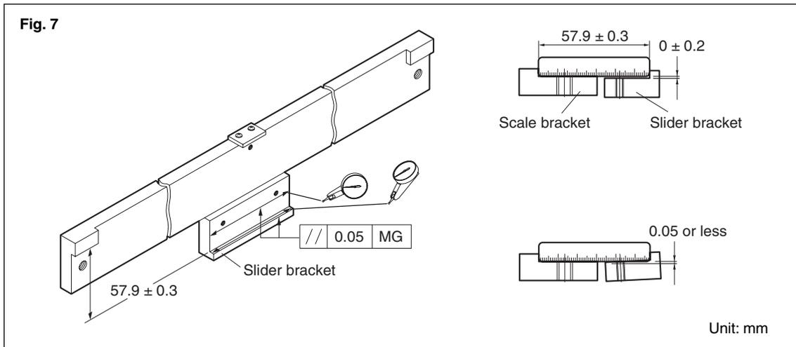
3. Bring the scale into contact with the stop surfaces and install.
